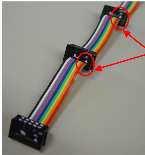
Fit the triangle-mark of the connector and the color of the flat cable together if you crimp the connector to the halfway of the flat cable.
