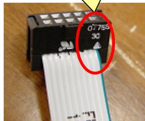
Fit the triangle-mark of the connector and brown cable core together if you have rainbow-colored type of flat cable.
