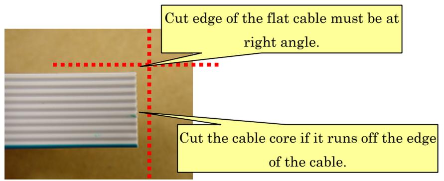
It is necessary to use industrial tool for crimping connector to flat cable. Commercial available vise or crimp tool suffices for it.
