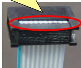
When you have crimped the connector to one side of the flat cable, next, crimp it to the other side. After making the cable, connect the CPU board and the extension board like the pictures below. (For reference of extension board, LED extension board "VS-IX004" is in the pictures below)
