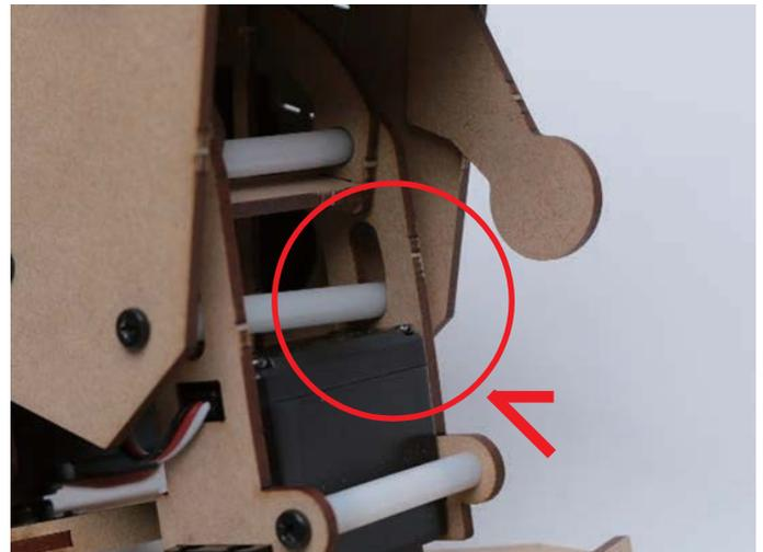
If the feet touch each other or spacer links hit the edge of the hole, the servo horn is determined to be misaligned. Please reattach servo horn to the axis of the servo motor. Little misalign is no problem but please just make sure that feet do not touch each other as well as spacer links do not hit the edge of the hole
