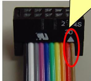
Fit the back side of the connector and the cut edge of the cable together.
