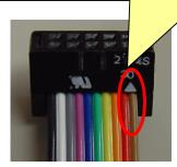
Fit the back side of the connector and the cut edge of the cable together.
