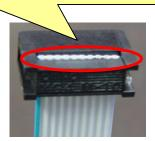
When you have crimped the connector to one side of the flat cable, next, crimp it to the other side. After making the cable, connect the CPU board and the extension board like the pictures below. (For reference of extention board, LED extension board "VS-IX004" is in the pictures below)
